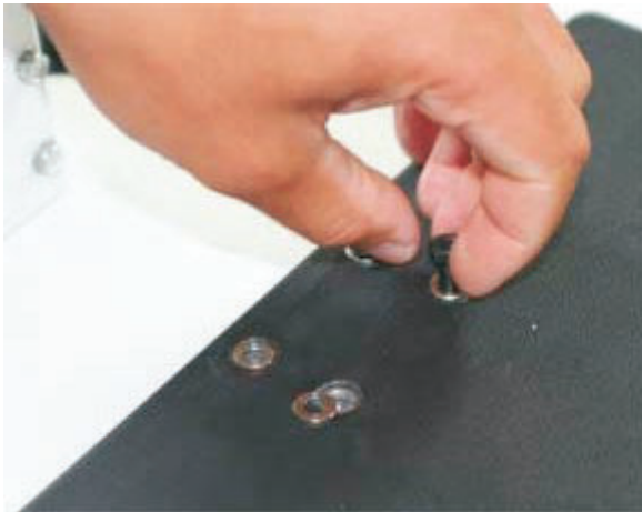
Figure 10. - Remove the four hex head screws from scale platform
